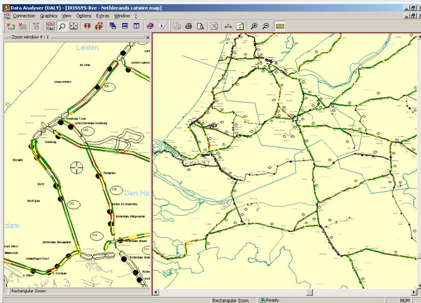
Computer maps of the route network allow demonstrative area researches. Any measuring data can be displayed right beside the tracks in a range of ratings. Faults in the network strike immediately. For detailed research, maps of particular areas can be imported via Autodesk Map® into IRISSYS®.
